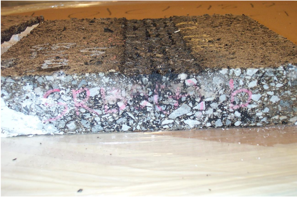
Figure C3 SR135 after Purwheel Testing
