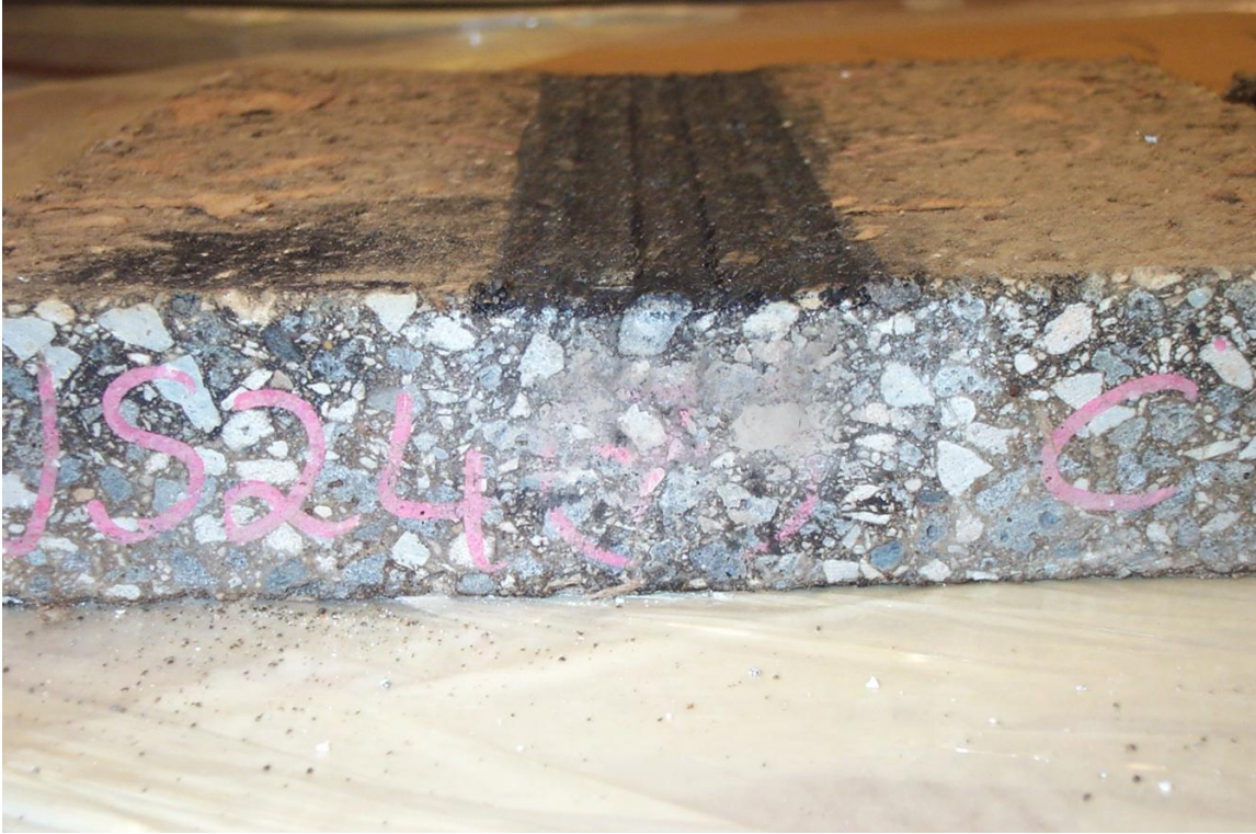
Figure C1 US24 after Purwheel Testing
